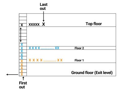
Total time (T) for evacuation = time for first occupant on floor 1 to leave building + delay until last occupant can move + time for last occupant to leave building (this needs thinking about).
