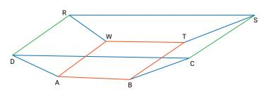
Figure 1 Diagram of empty rectangular dam
