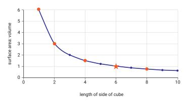
Create a graph plotting the ratio for blocks with lengths from 1 to 10. This shows that smaller cubes have higher surface area/volume ratios than larger cubes. That is, smaller cubes have a greater surface area through which to lose fluid relative to the volume of fluid they have to lose. Smaller cubes will lose fluid at a greater rate than larger cubes.
