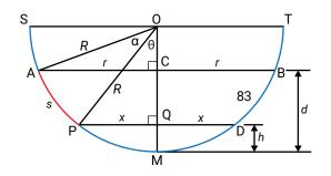
Figure 1 Cross-sectional diagram of a partly full dam
