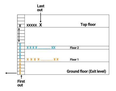
Total time (T) for evacuation = time for first occupant on floor 1 to leave building + delay until last occupant can move + time for last occupant to leave building (this needs thinking about).
